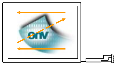
Fig. 2 Reverse scan (Pin4, DPS = High)
